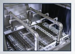
Adjustable spray nozzles give you the ability to clean a high-volume of parts by a continuous, flow-through wash section with 360-degree part coverage.
